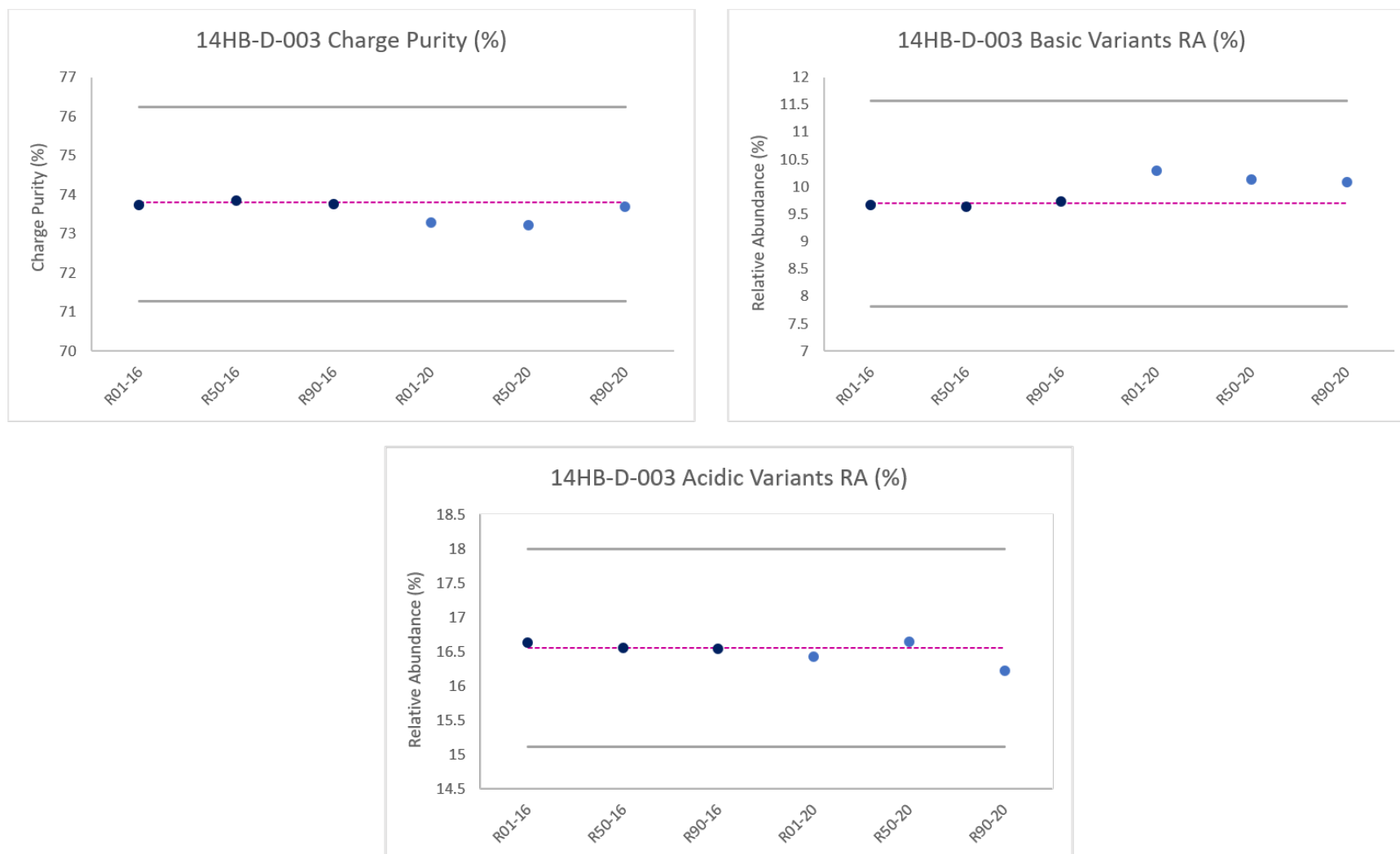
Figure 17. Charge heterogeneity control charts using capillary zone electrophoresis for lot 14HB-D-003. Initial certification (0y) data is shown in dark blue and 5YSV (5y) in light blue. Pink dotted line corresponds to the non-certified value assigned in the original 2016 certification. Control limits set at \pm 3u_c (grey bars).
